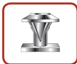
Flares rolled out above die bar.
